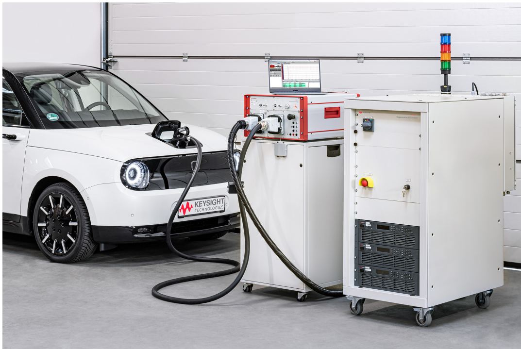
Figure 6. The electric car (above left) can be tested to ensure it works with different types of charging stations simply by using an emulator (middle) and a regenerative bidirectional power supply (right).
